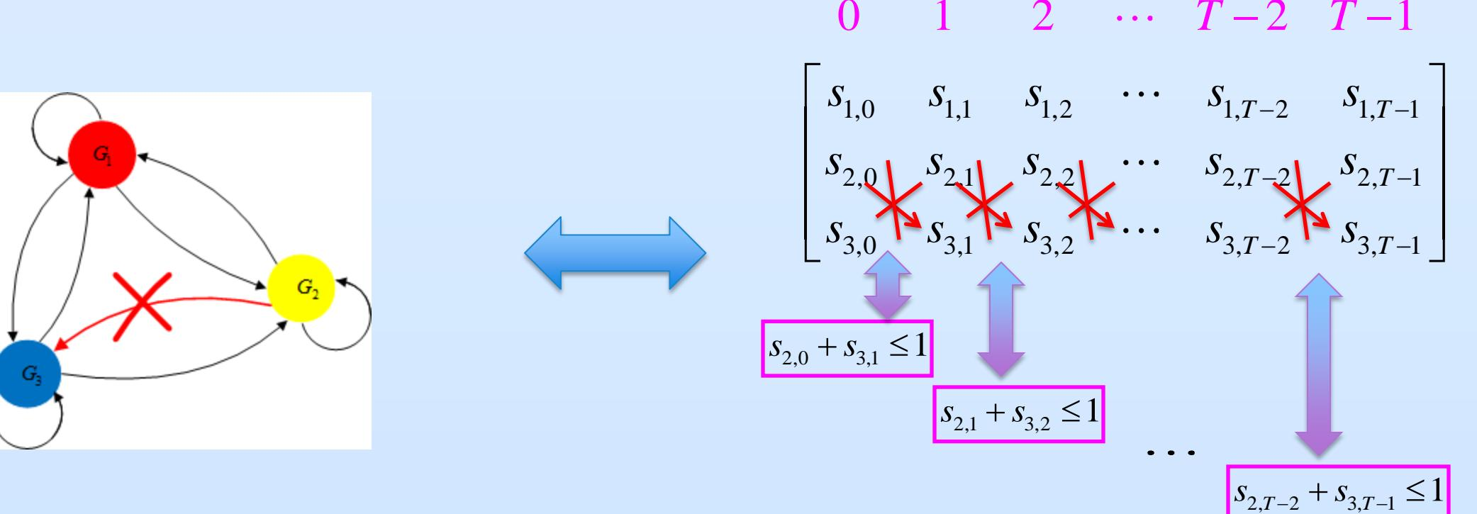
The structural constraints are imposed as linear inequality constraints on the indicator variables
