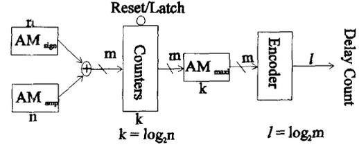
Fig. 4. A memory-based architecture for two bit correlation.
