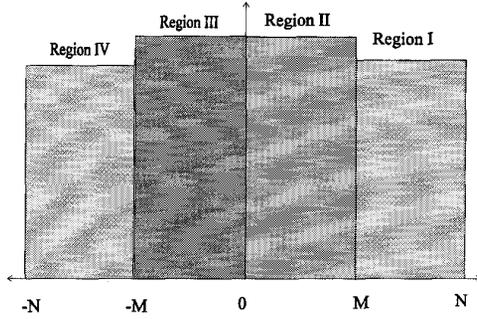
Fig. 2. Two bit partition of signal/noise regions.
