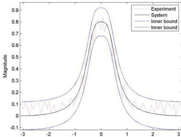
Fig. 2. Inner bounds for the consistency data set (dashed) vs. experimental outcome (dotted) and real system (full).
