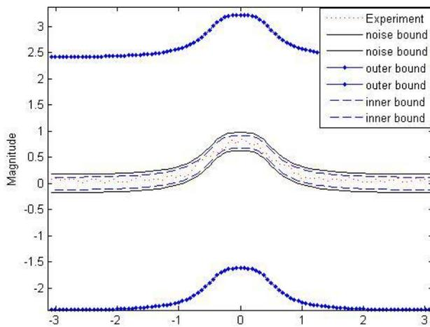
Fig. 3. Inner (dashed) and outer (dash-dot) bounds for the consistency data set vs. experimental (dotted) and noise bounds (full).
