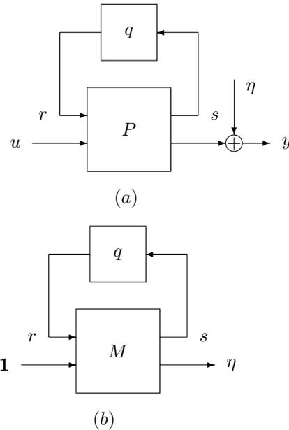
Fig. 1. (a) Robust Parametric Identification Set-up. (b) Equivalent Formulation.
