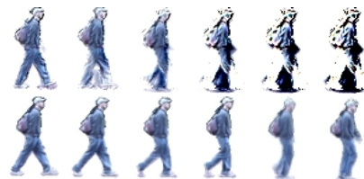
Figure 1. Generated walking sequence after the learning step, t = 38, 40, \dots, 48 . Top: from constant acceleration dynamics; Bottom: from dynamics identified using robust estimation
