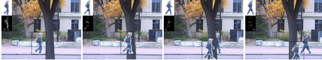
Figure 2. Dynamic appearance and occlusion by a background object, t = 60, 75, 90, and 105 . The white box is the predicted appearance and the black box is the probability map based on the predicted appearance.
