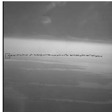
**Figure 7. Tracking algorithm applied on an image sequence with the target aircraft (marked by a rectangle) translating from right to left at a distance of 3 nmi (5.4 km).**
