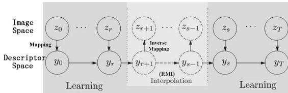
Figure 1. A general model for video inpainting by nonlinear dimensionality reduction, rank minimization and nonlinear reconstruction.  $z_t$  and  $y_t$  represent the appearance in the image and descriptor space respectively.
