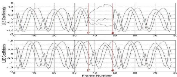
Figure 4. Top: low dimensional (3-D) representation of a walking sequence on an LLE manifold; frames 37-49 have occlusion. Bottom: Descriptor sequence interpolated via rank minimization.
