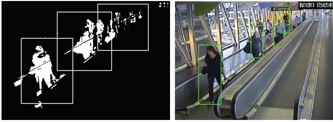
Fig. 4. Human detection example using MoG foreground detection to reduce computational complexity.
